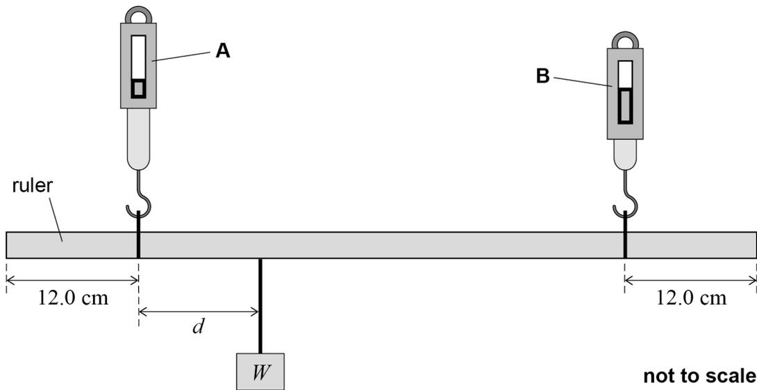
The reading on **A** is  $0.82\text{ N}$  and the reading on **B** is  $0.62\text{ N}$ .
